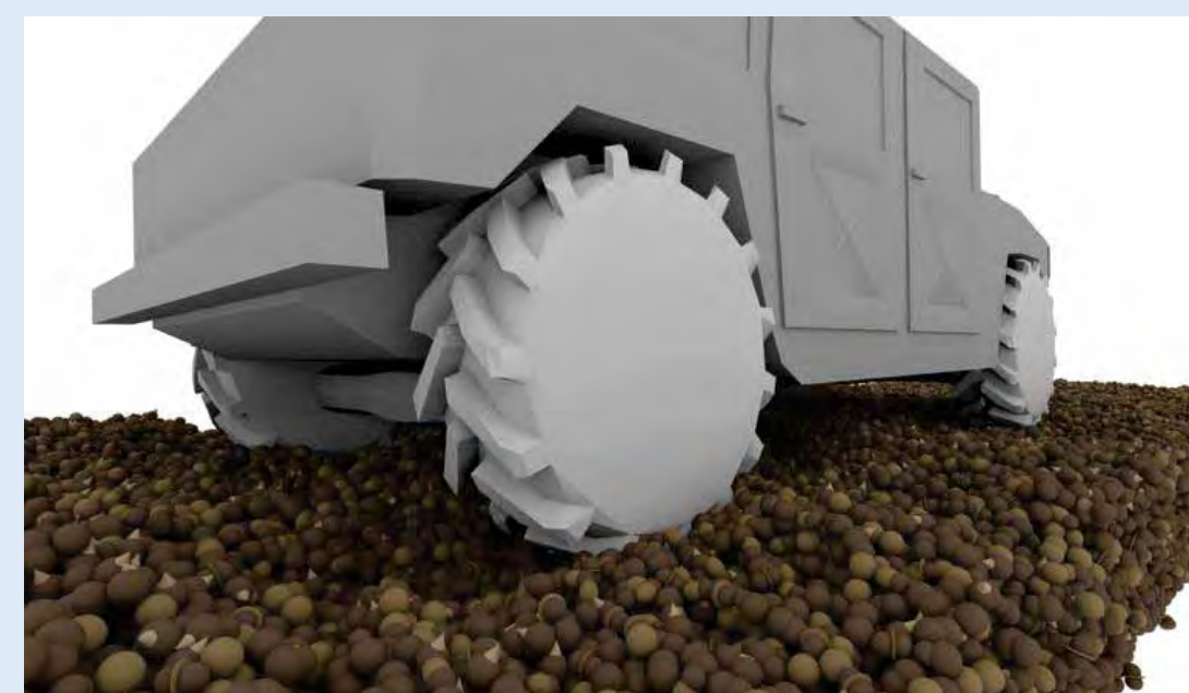
Humvee tire on granular soil.
